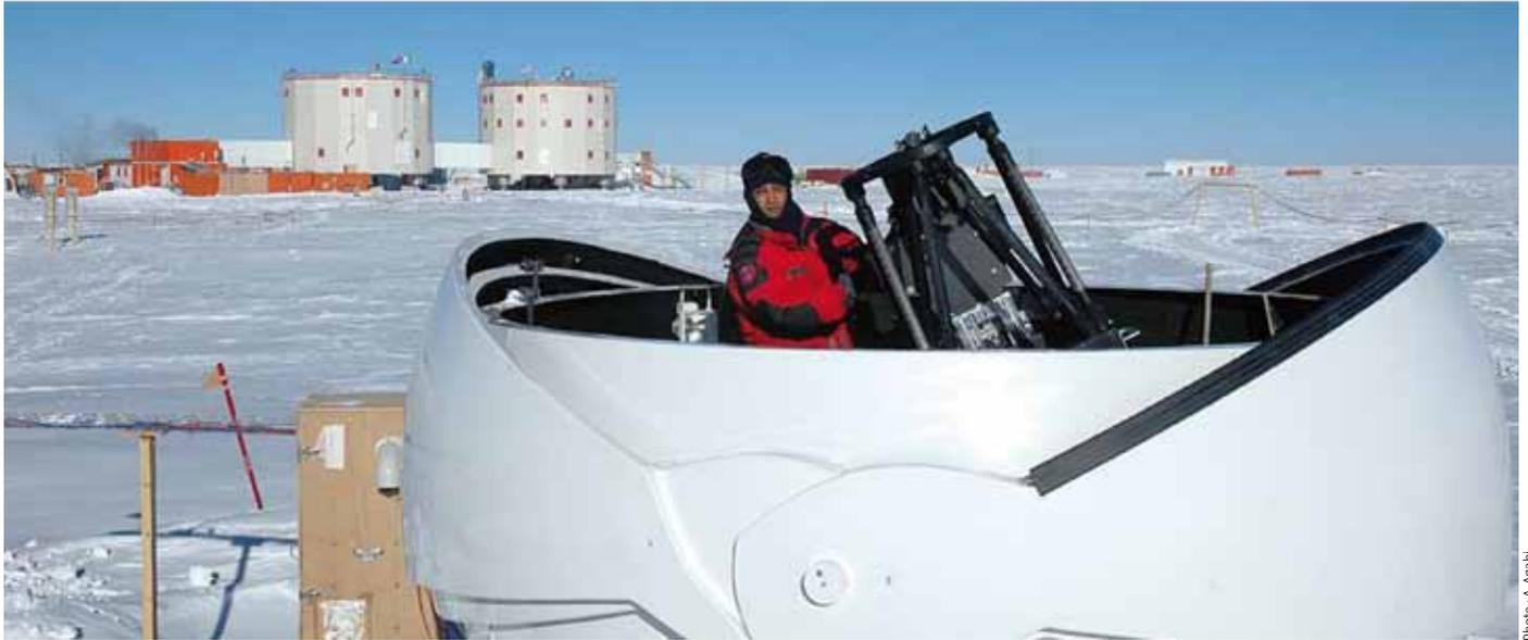
The 40cm planetary transit telescope ASTEP
