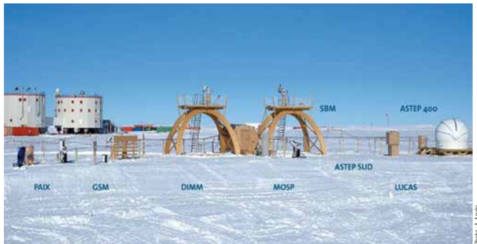
The Concordia station and the site testing equipment
