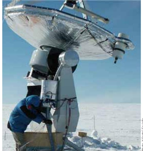
The 2.5m millimetre-wave telescope COCHISE
